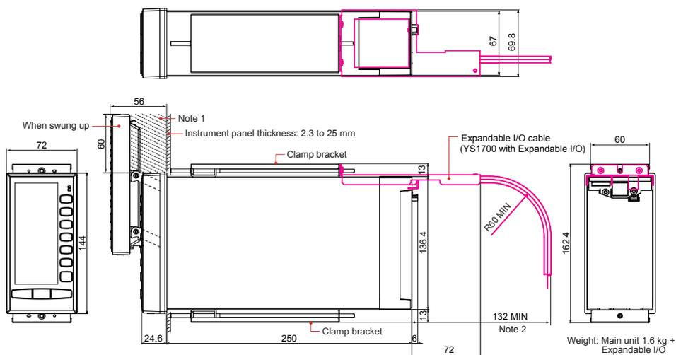
Weight: Main unit 1.6 kg + Expandable I/O Cable 320 g
