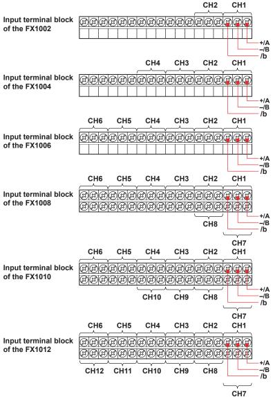
For TC input, use shielded compensating lead wires for wiring.
